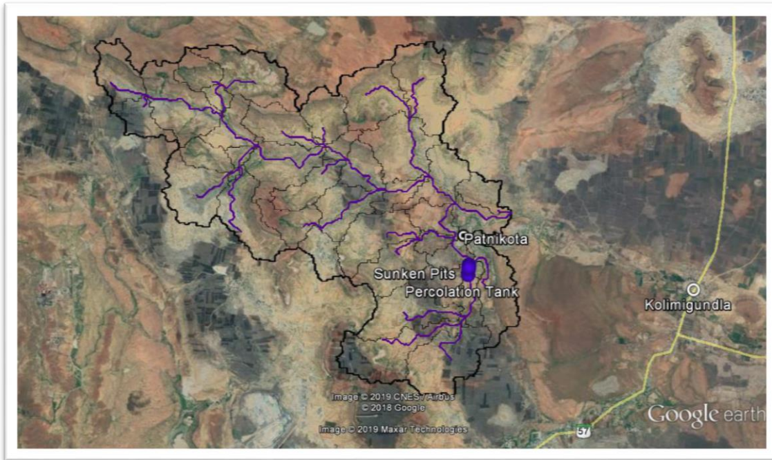
Figure 17. Spatial distribution of streams and water conservation structures created in the watershed.
