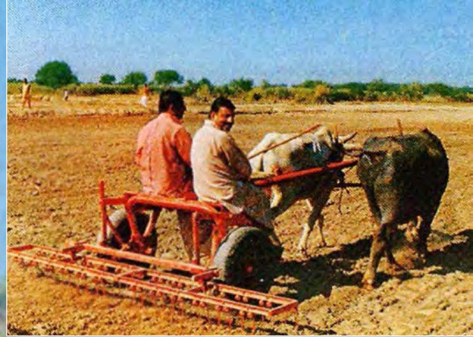
Bullock driven tropicultor allows the farmer to perform many operations at once
