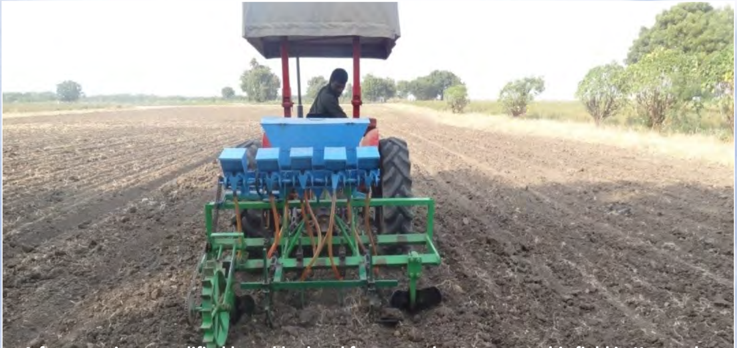
A farmer using a modified broad bed and furrow maker to prepare his field in Karnataka
