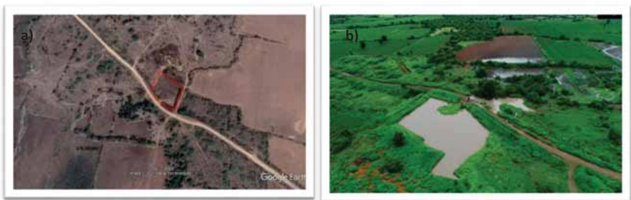
Figure 20. Percolation Tank 2 and Sunken pits created on a stream in the watershed a) before and b) after rain water.
