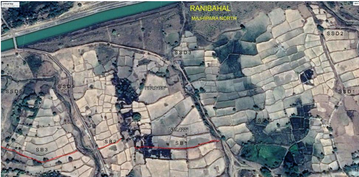
Figure 29b. Proposed water conservation structures in Ranibahal village, secondary bunds SB 1 & 2.
