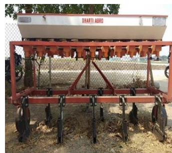
Figure 4.18: Zero till multi crop bed planter.
