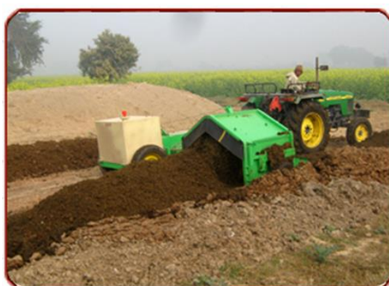
Figure 3.2: Compost heap turning over machine
