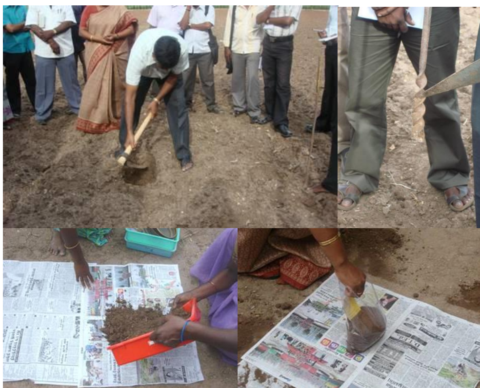
Figure 2.3: Equipment for soil sampling- Screw augur, Plastic tray, Polythene bag, label and marker
