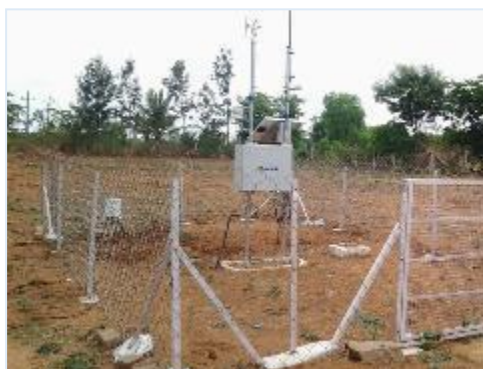
Figure 15 a): Runoff setup at Haralakatte village in Tumkur; downloading DIVER data; automatic weather station.
