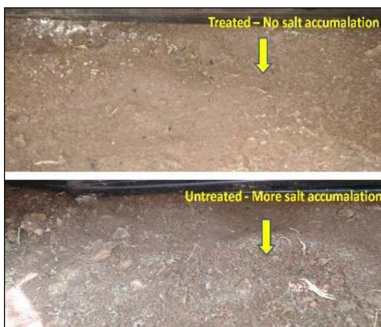
Figure 21: Impact of magnetic water conditioner in field.
