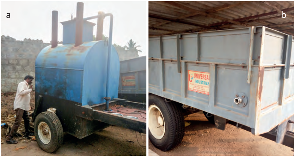
Figure 10.6. The boiler parts: (a)The steamer and (b) the turmeric container.
