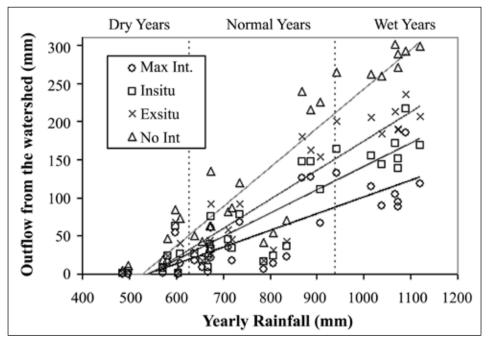
Figure 2. Rainfall-Runoff relationships for the four different water management scenarios in a micro watershed project at Kothapally located in the SAT zone of Southern India.
