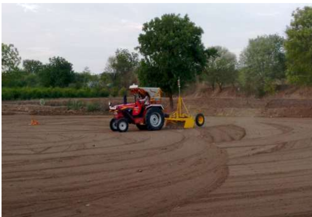
Figure 99. Laser land leveler in operation in Inchageri village.
