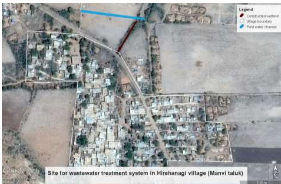
Figure 72. Location of village, proposed constructed wetland, and existing field water channel.
