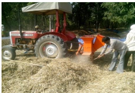
Figure 6.1.1.1: A tractor operated shredding machine used for shredding crop & plant wastes
