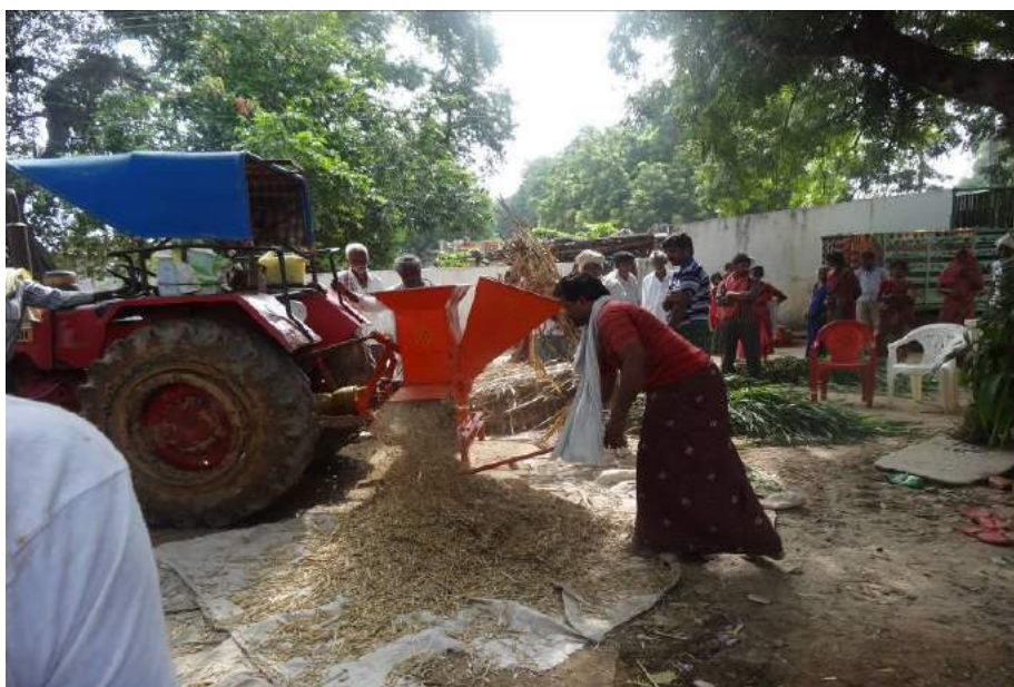
Figure 3.2.4.1. Shredding machine demonstration for chopping-off biomass in Porumamila village, Kadapa district.
