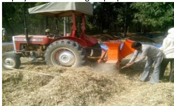
Figure 4.1.1.2. Shredding machine for chopping biomass for aerobic composting
