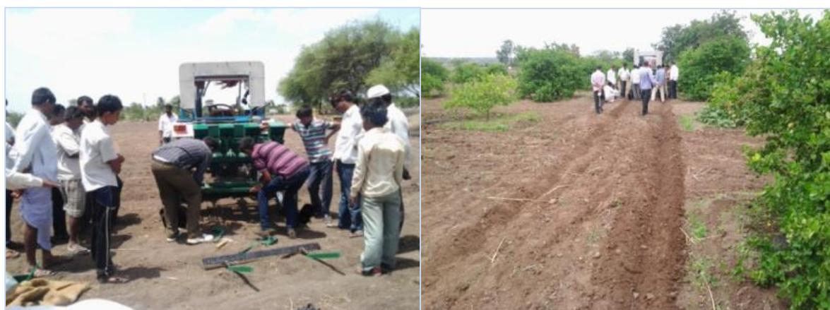
Figure 10. Tropicultor attachments; Sowing with Tropicultor; Farmers checking seed depth and spacing
