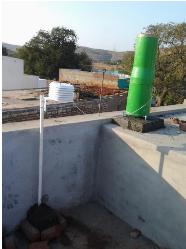
Figure 7. Rain gauges have been installed in the project area.
