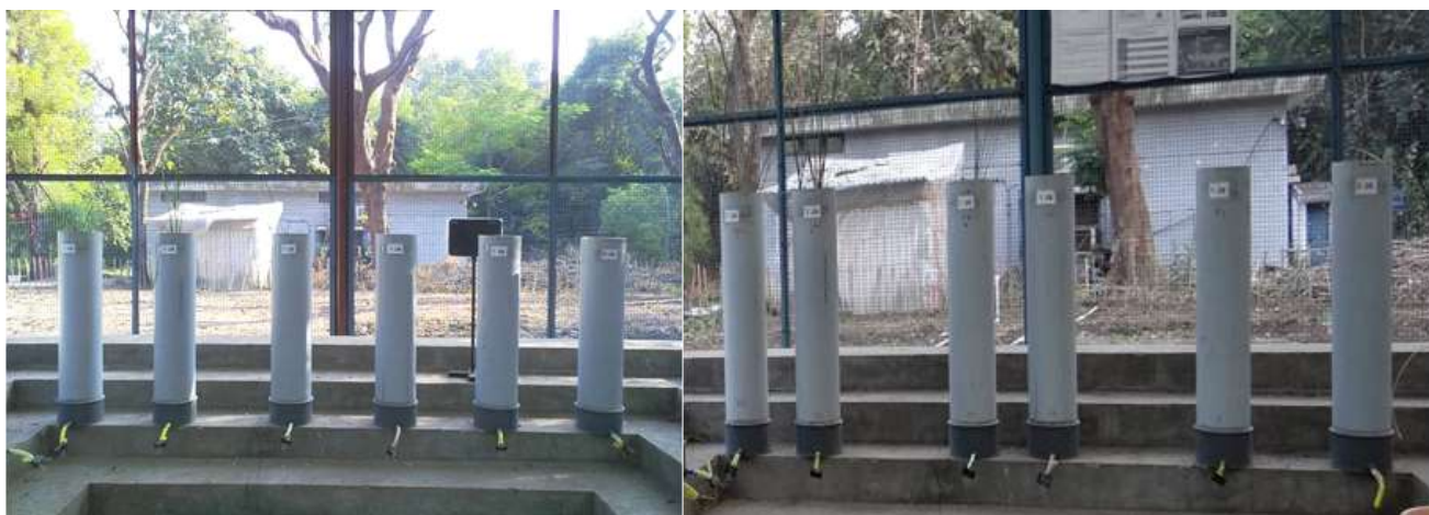
Figure 2-2. Column lysimeter experiments to study the removal trend of pollutants, clogging and biofilm formation installed at CSIR-NEERI, Nagpur
