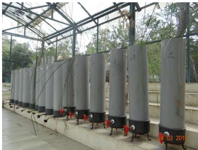
Figure 2-5. Column lysimeter experiments to estimate the removal efficiency of parasites and pathogens using different substrate materials and vegetation
