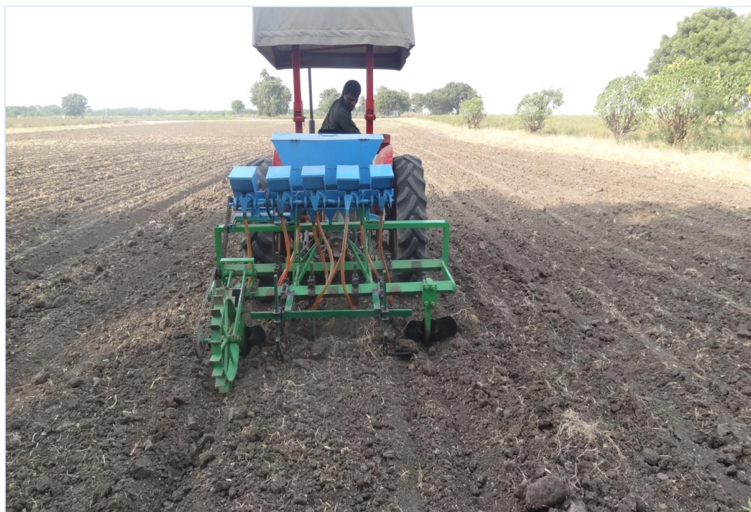
Figure 4. Prototype seed drill cum BBF maker in Bijapur
