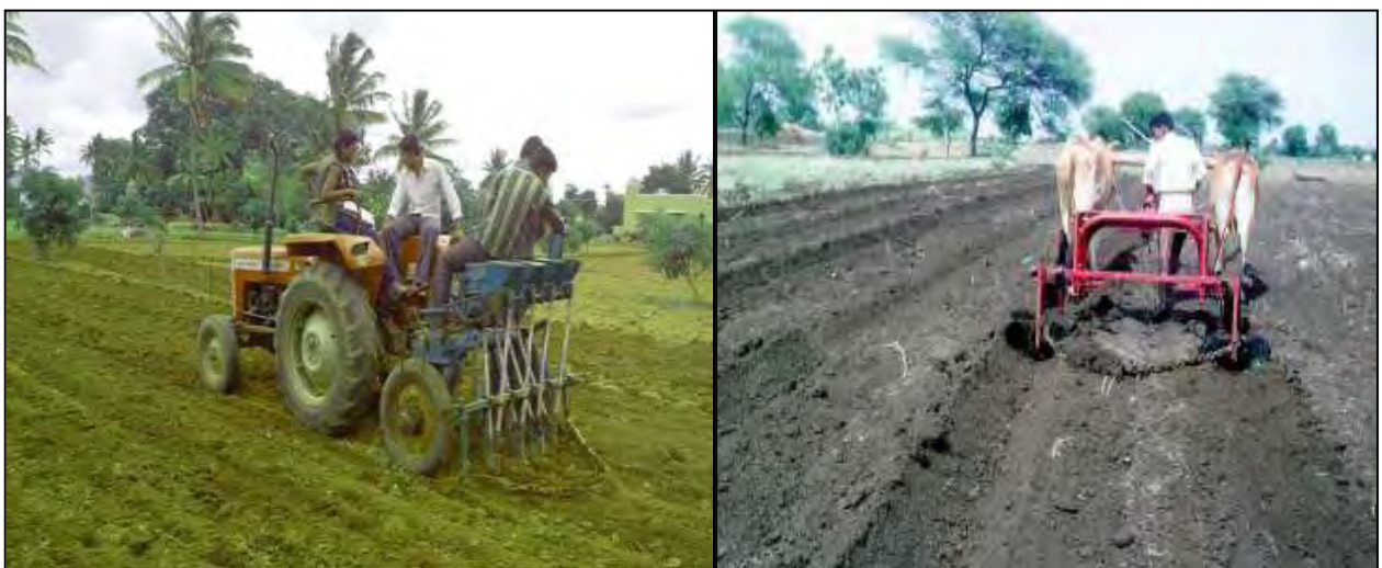
Figure 5. Line sowing of Ragi crop using tropicultor in Kolar (L); BBF shaping with Tropicultor.
