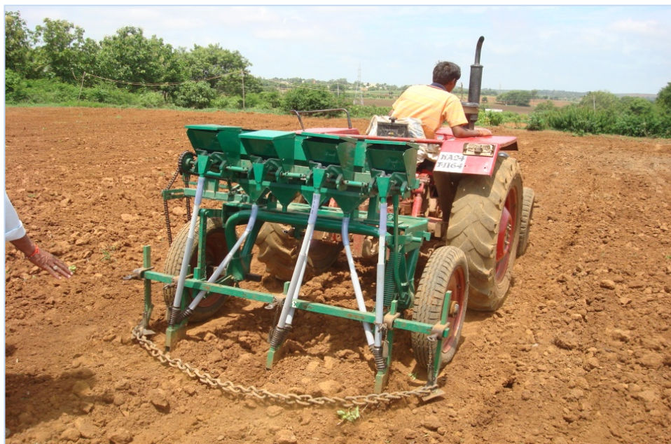
Figure 3. Applying fertilizer and seed at a time with tractor mounted with a Tropicultor in Kottur watershed, Dharwad
