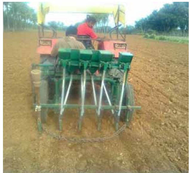
Figure 4b. Applying fertilizer and seed at a time with Tractor mounted Tropicultor in Kottur watershed, Dharwad
