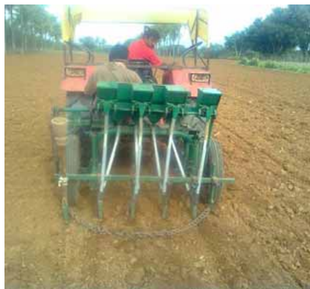
Figure 4b. Applying fertilizer and seed at a time with Tractor mounted Tropicultrator in Kottur watershed, Dharwad
